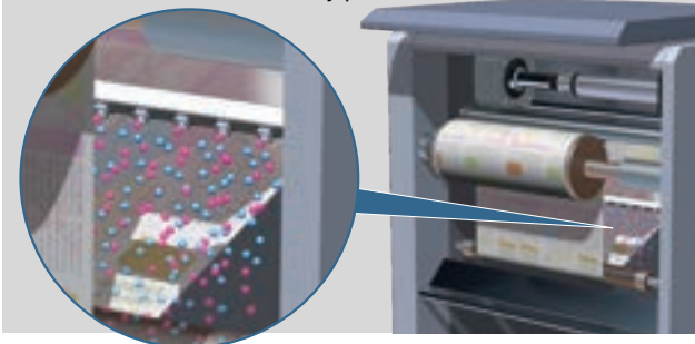
Static neutralisation of a rotary press
