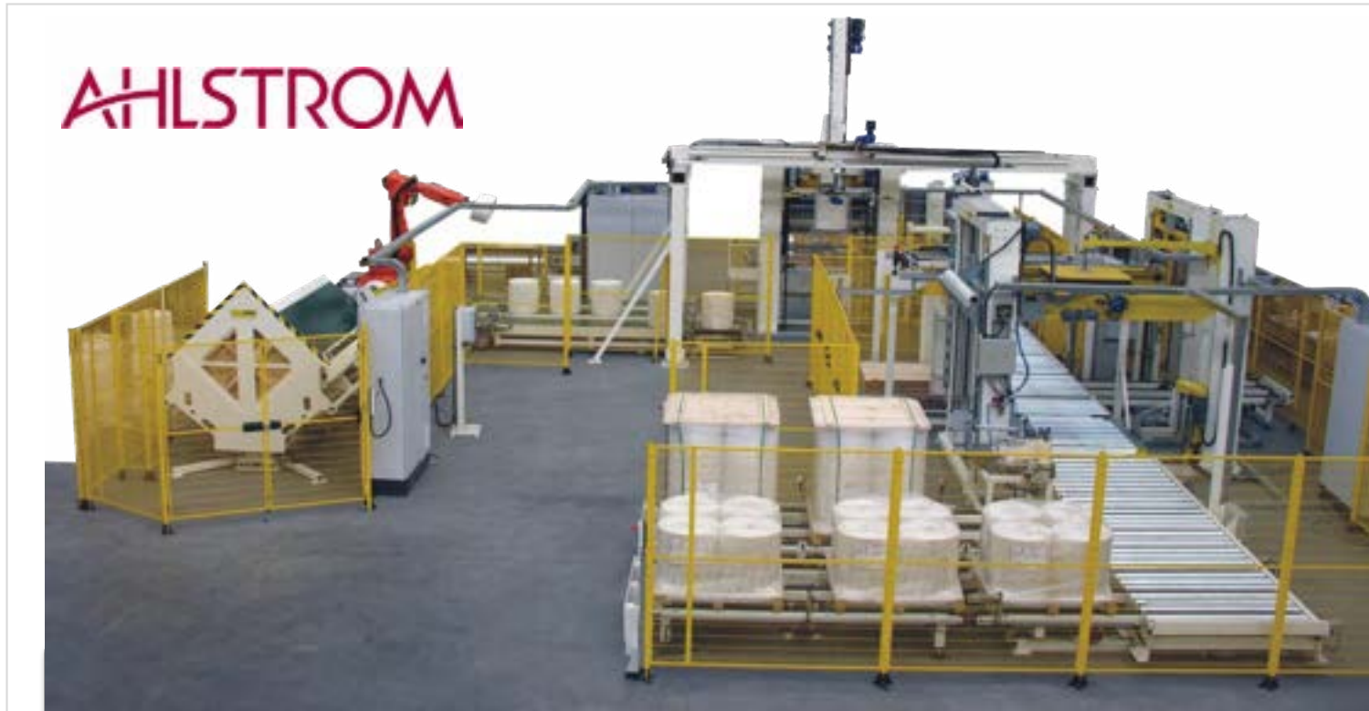
Packaging and palletizing installation for non-woven materials
