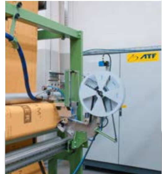
Liner application with hot melt
