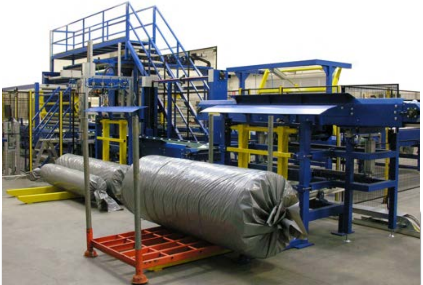
Packaging machine for big rolls - Ends closing with ultrasound
