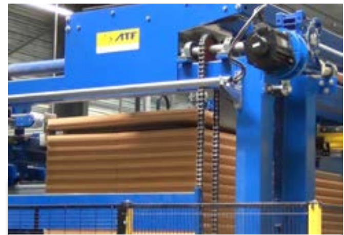
Stacking of the milled panels
