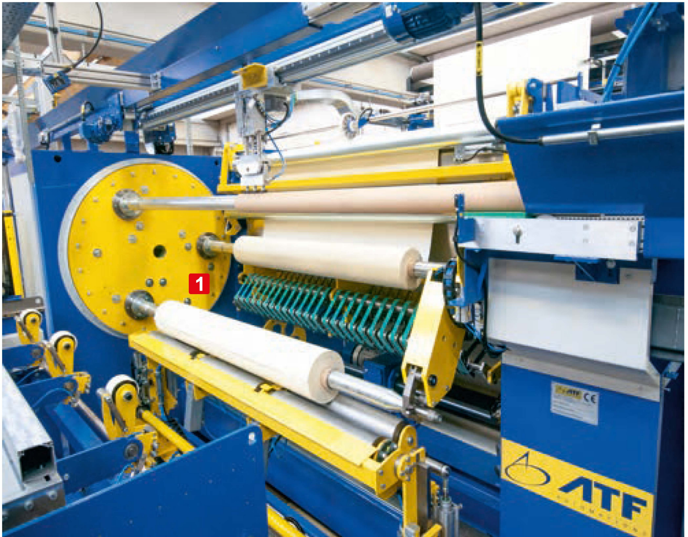
Automatie winder with integrated packager
