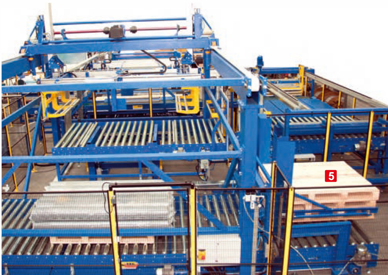
Palletizing plant for heavy rolls (PVC -TPO)
