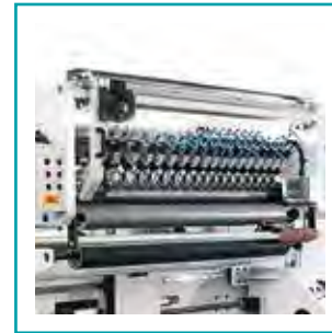
6 Comfort kit can be added to improve the accessibility to the slitting section, while maintaining the compact configuration.
