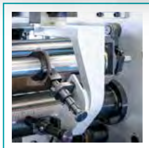
12 MTS bar for knives positioning aid
